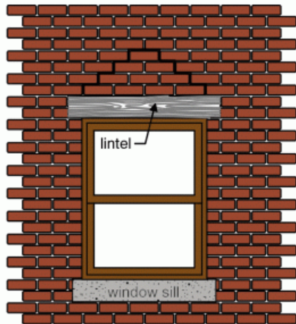
cracking caused by deterioration of wood lintel
