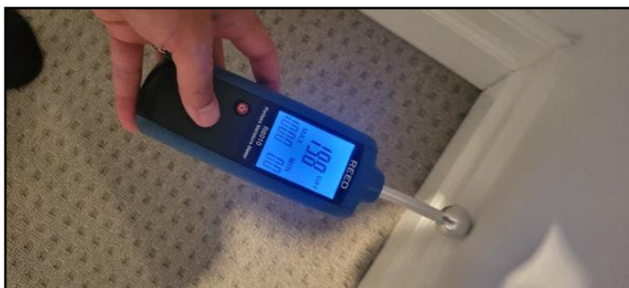
82. Moisture meter results
